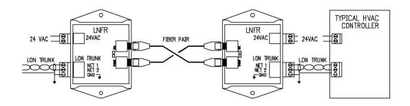
The LNFR single channel fiber repeater is used in a point to point application to extend the physical twisted pair network up to 2.5 km. The LNFR acts as a repeater only, and is completely transparent to the network. Any communication received on the near side of the free topology network will be propagated to the far side via fiber optic cable, where the twisted pair signal will be regenerated on the far side of the network.
